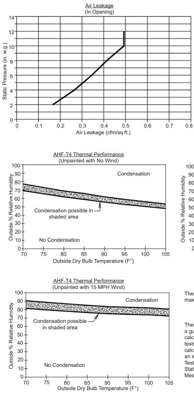
Air leakage chart is based upon independent air leakage tests conducted by Architectural Testing Laboratory. The out-opening model of a 24" x 60" AHF-T4 was tested. Tests were in accordance with ASTM E 283-91 "Determining the Rate of Air Leakage through Exterior Windows, Curtain Walls, and Door under Specified Pressure Differences Across the Specimen". Arrow United Industries recommends using out of opening doors for draw through applications and in opening (IO) for blow through applications.
