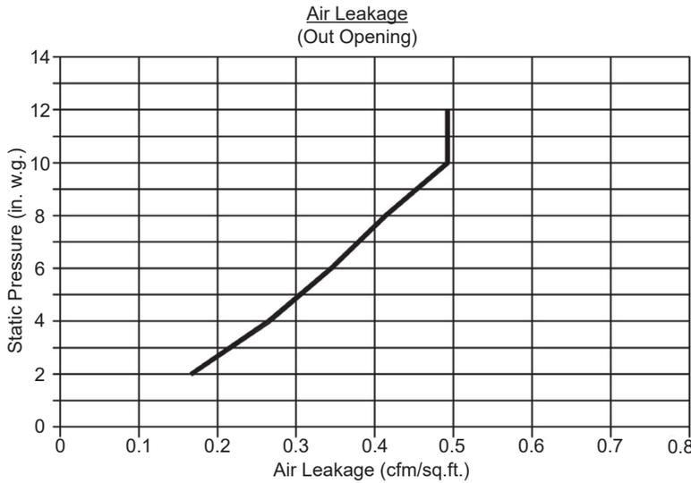
Air leakage chart is based upon independent air leakage tests conducted by Architectural Testing Laboratory. The out-opening model of a 24" x 60" AHFT40 was tested. Tests were in accordance with ASTM E 283-91 "Determining the Rate of Air Leakage through Exterior Windows, Curtain Walls, and Door under Specified Pressure Differences Across the Specimen". Arrow United Industries recommends using out of opening doors for draw through applications and in opening (IO) for blow through applications.
