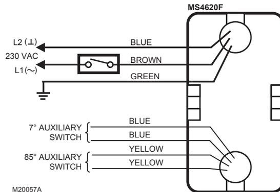
Fig. 9. Typical 230 Vac wiring (MS Series).
