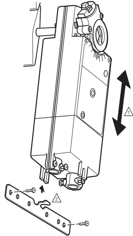
1 ENSURE THAT MOUNTING ASSEMBLY PREVENTS ACTUATOR ROTATION AND ALLOWS ACTUATOR TO FLOAT ALONG INDICATED AXIS. WHEN TOO TIGHT, THE RESULTING BINDING CAN DAMAGE THE ACTUATOR OR REDUCE TORQUE OUTPUT.
