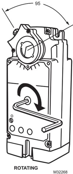
Fig. 6. Manual positioning.
