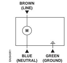
**NOTE:** Wire the 230 Vac actuator with a 230 Vac line with respect to neutral and connect the ground lead for proper protection of the actuator. Any other connection such as phase-to-phase, can damage the actuator.
